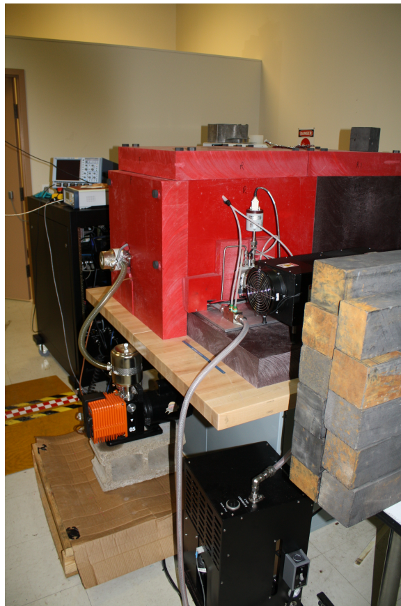
Figure 28. Exterior view of the D+D testing environment. The red blocks are borated polyethylene for blocking neutrons from escaping the generator assembly and penetrating into the surrounding rooms.
